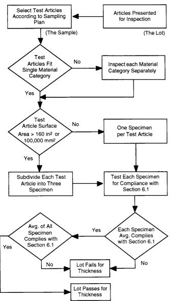
FIG. 3 Coating Thickness Inspection Steps
