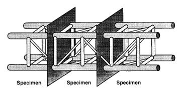
Note 1—Each specimen comprises nominally one third of the total surface area of the article. A minimum of five measurements should be made within the volume of each specimen, as widely dispersed within that volume as is practical, so as to represent as much as possible, the general coating thickness within that specimen volume.
