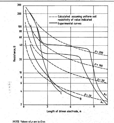
Figure 5 — Calculated and experimental curves of resistance of 12.5 mm diameter driven rod electrodes
