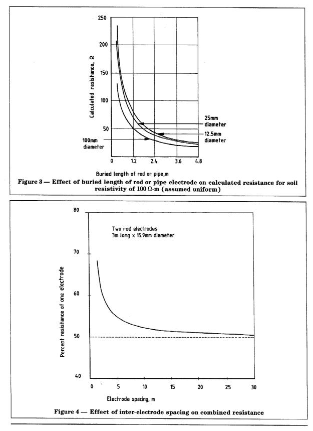
The combined resistance of rod electrodes in parallel For three rods placed in an equilateral triangle, or in  $R_{n}$ , expressed in ohms ( $\Omega$ ), can be obtained from the following equation:
