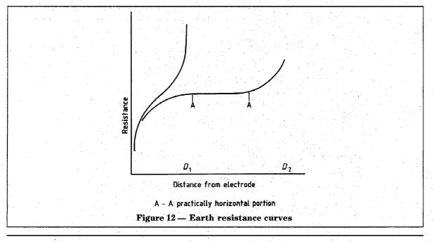
electrode system, ultimately found to have a resistance of  $0.05 \Omega$ , it was necessary to place Y 700 m away and the horizontal section of the curve was found for potential electrode distances of 70 m to 100 m.
