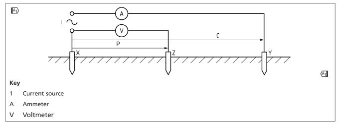
NOTE 2 To avoid polarization effects, commercially available testers commonly employ an alternating square wave current, at or near power frequency. A slight offset from multiples of the utility frequency enables the tester to base its reading on its own signal, without interference from utility harmonics.
