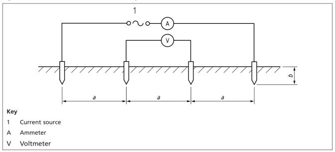
The resistivity found applies to soil depth b, so by repeating the measurement with different values of a, the average resistivity to various depths may be found and the results indicates whether any advantage is to be gained by installing deeply driven electrodes in order to reach strata of a lower resistivity.
