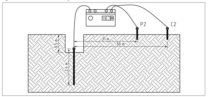
NOTE This method is particularly useful if HV and LV electrode systems are to be separated.
