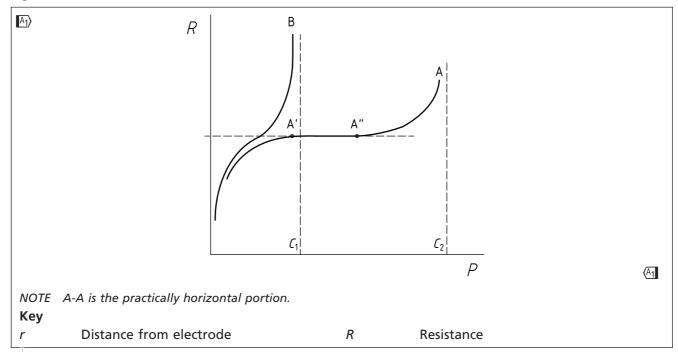
If the characteristic shape of the graph is not achieved, the current probe should be moved farther out and the procedure repeated. In many instances space and time constraints make a level graph section impractical or difficult to achieve and alternatives techniques such as such as the slope method (10.3.7) or the 61.8% (10.3.3) method may be used.
