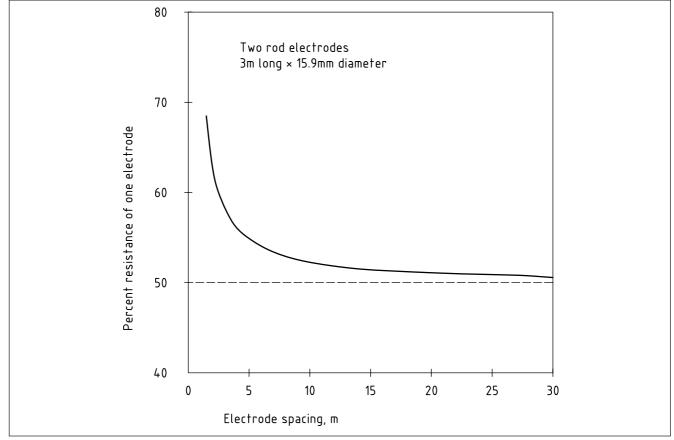
Figure 14a Effect of inter electrode spacing on combined resistance
