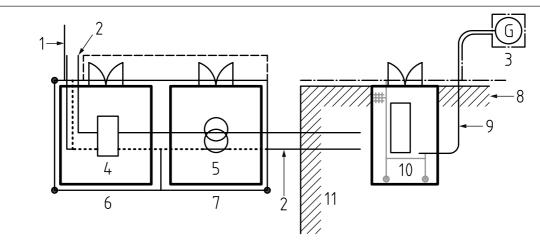
NOTE Typical switchroom layout with external HV supply. Supply companies' preferred method. Key
