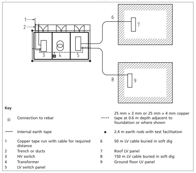
Figure A.6 External HV/LV interface and generator backup
