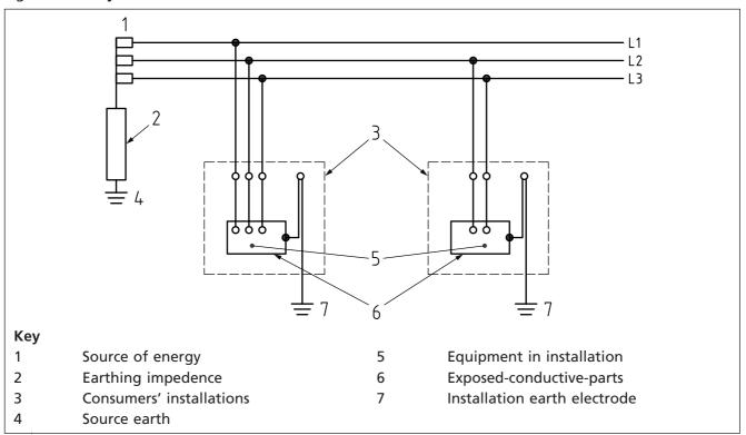
Generally an IT system would be chosen in locations such as medical centres and mines where the supply has to be maintained even in the event of a fault, and where the connection with earth is difficult (for example a mobile generator).
