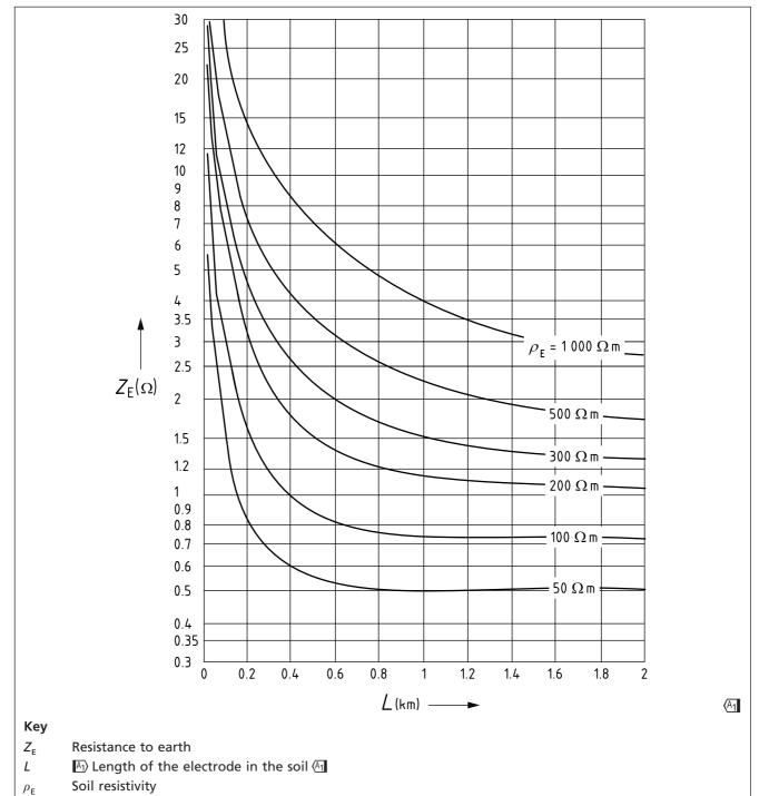
Impedance to earth of horizontal earth electrodes buried in homogeneous soil Figure 14
