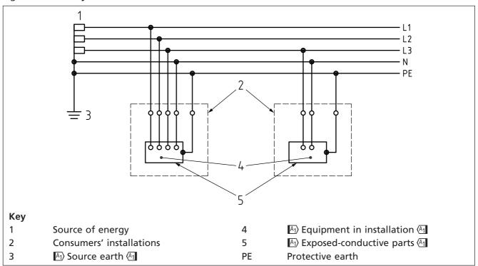
A TN-S system has a particular disadvantage that in the event that the protective conductor becomes open circuit, there is no indication that a fault has occurred and installations can unknowingly be left without an earth. In the event of an earth fault all of the exposed-conductive-parts within a consumer installation may be raised to a hazardous potential. Earth fault protection devices will not operate as there will be no flow of current to earth.
