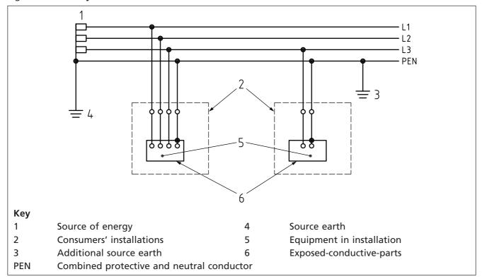
The need for multiple earth connections is because if the neutral becomes open-circuit for any reason, the exposed-conductive-parts will rise to line to earth voltage in the case of single-phase connections and a value up to line to earth voltage in the case of three-phase connections, depending on the degree to which the load is unbalanced.
