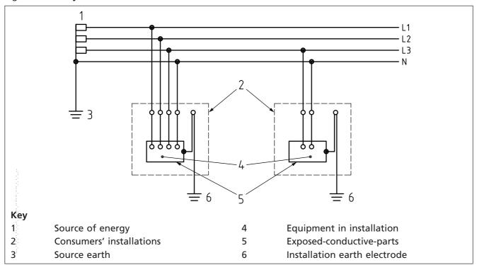
In the TT system the earth fault loop impedance is generally high as the fault path includes the earth electrode resistance of the supply and the earth electrode resistance of the consumer's installation.
