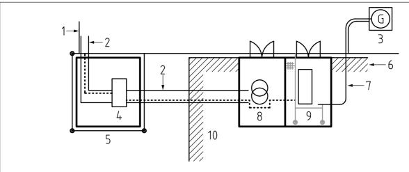
NOTE Typical substation layout with external HV switch. Supply companies' preferred method.
