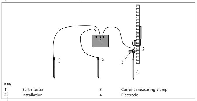
This test may be used where an electrode is connected to an Earthing system with a much lower overall resistance than the electrode in question. In effect this test may be used to measure the loop impedance of the electrode under test and the rest of the earth system it is connected to.
