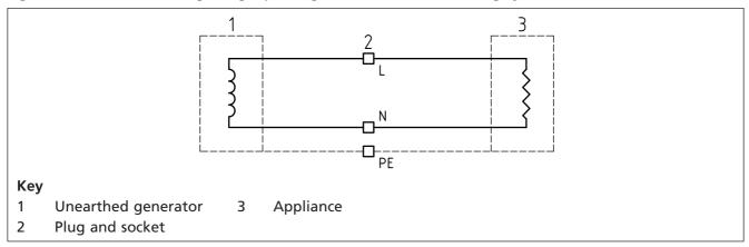
Cables, plugs, socket-outlets and cable couplers should be suitable for their environmental exposure. Cables should be a flexible type which includes a metallic braid or screen suitable for use as a protective conductor.
