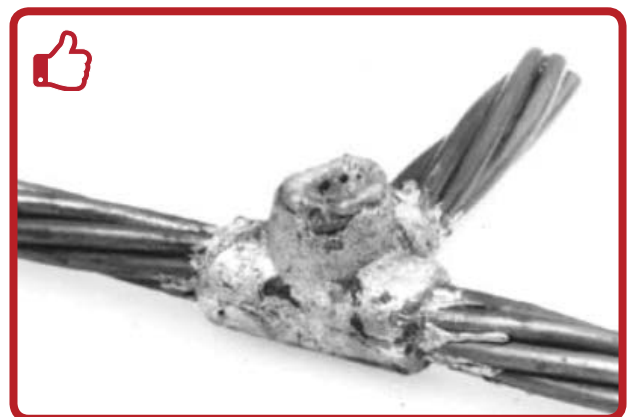
The presence of water/moisture in conductor strands or mold indicates that one or both were not properly dried. Although the riser is porous, the weld is solid. The degree of porosity is not sufficient to reject this connection.
