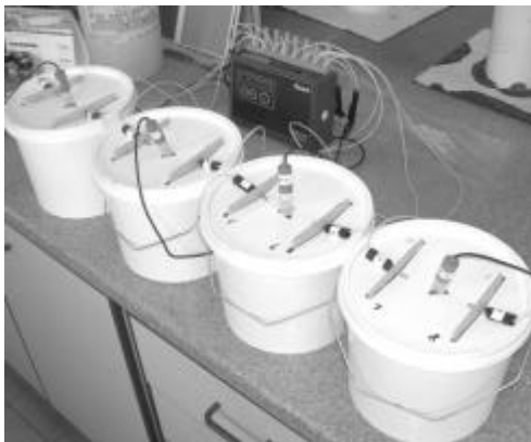
FIGURE 4 – Open circuit potential set-up
