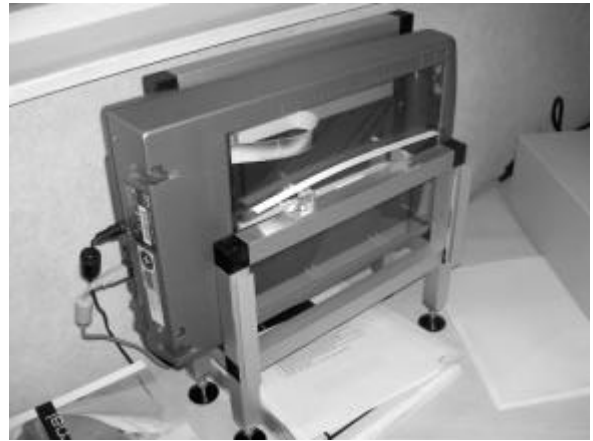
FIGURE 8 – Coated shim under test
